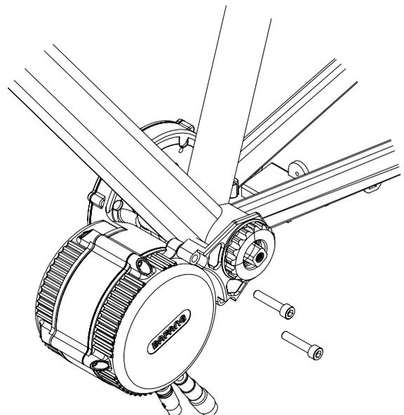
**4. Loosely screw in the 2x M6 Plate Bolts.**
