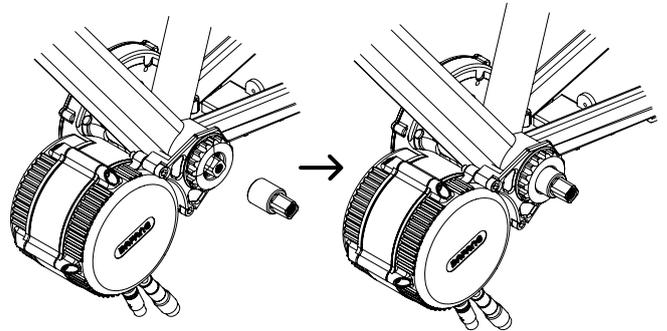
6. Grease the left side axle and slide on the Axle Extender.
