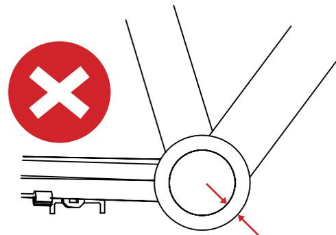
Carbon frames often have a lot of reinforcing under the BB shell of the frame. The motor cannot fit due to material thickness.
