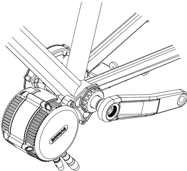
7. Grease the Axle Extender and slide on the disassembled left Buzz Bar.
