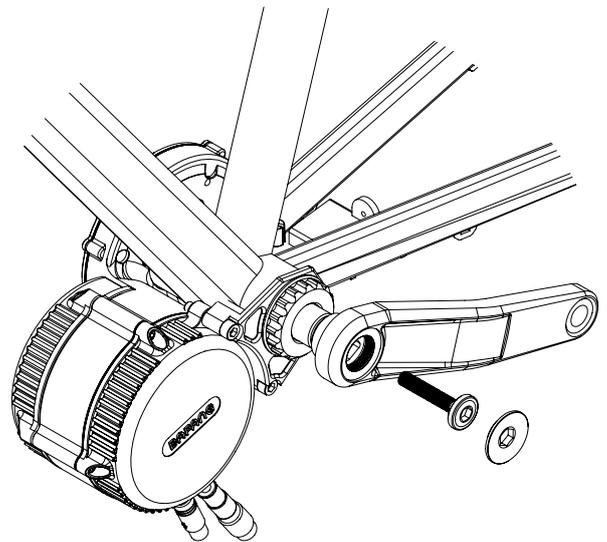
8. Using the Extender Crank Bolt tighten the axle extension assembly onto the motor and re-install the crank extractor.
