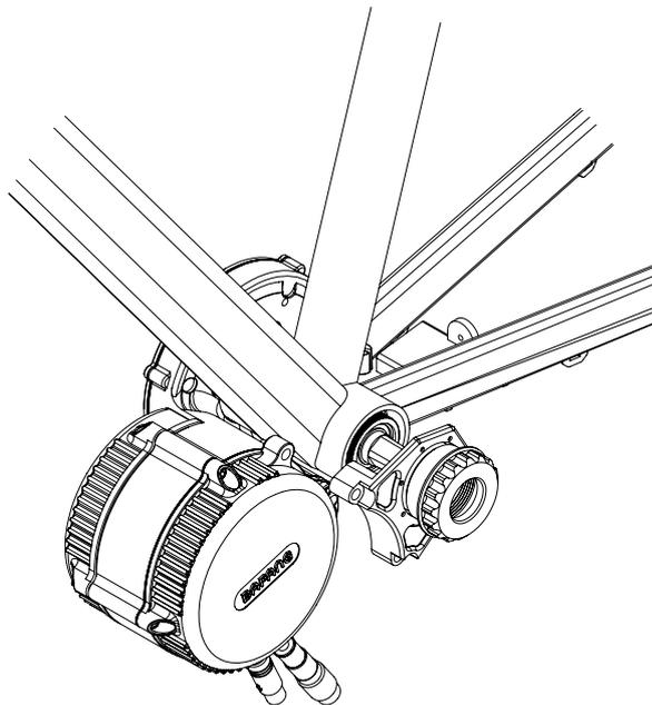
**3a. Grease the inside of the frame on the left side.**
