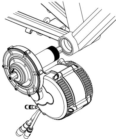
**2. Grease motor body shaft and slide through from the right hand side.**
