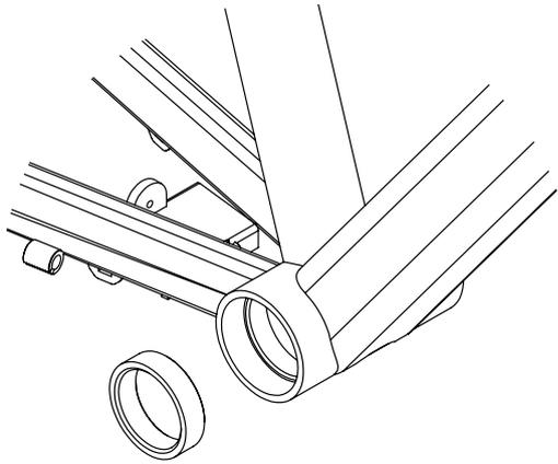
**1. Grease and press the Drive Cup into the right side of the frame. It must be pressed hard against the inner lip.**
